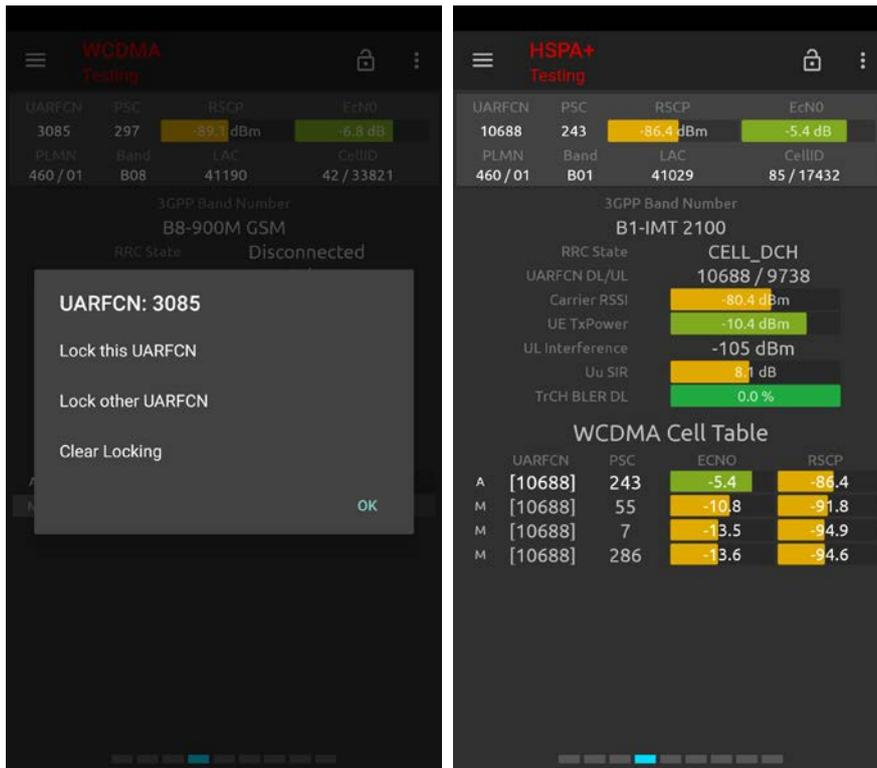
User can hold the cell table of UMTS and bring up the menu of this action. Pick the selected command and then take into effects. To clear all of the locking, tap clear locking and all of the locking will be disabled.
