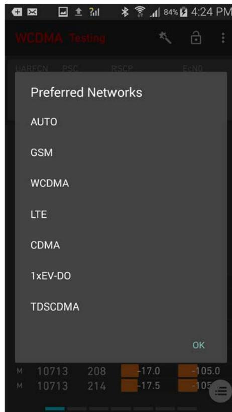
This function locks the device to a subset of its supported radio access technologies when in idle mode. The function does not have any effect on RAT selection in dedicated mode.
