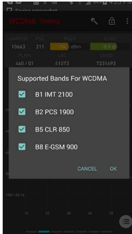
B1 IMT 2100 etc.: The device will be locked to the indicated subset of WCDMA bands.
