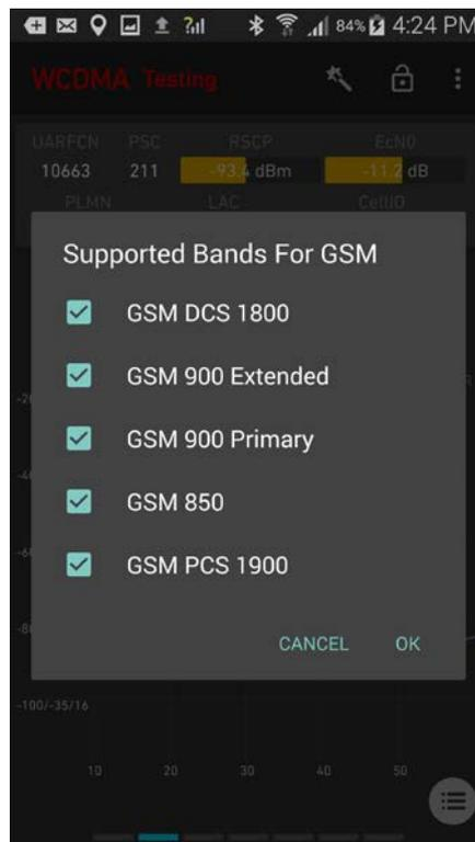
GSM 850, etc.: The device will be locked to the indicated subset of GSM bands.
