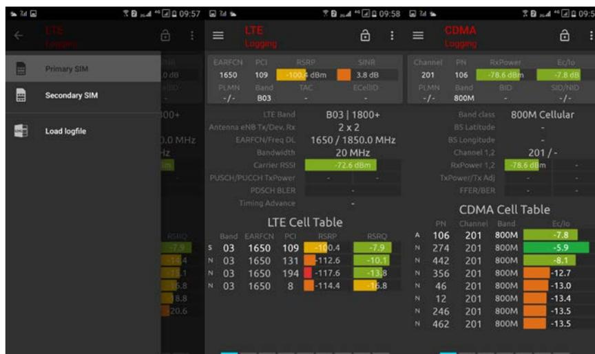
From the pictures, we have 2 SIM in one phone, in the previous version, the views are switching constantly from 1<sup>st</sup> SIM to 2<sup>nd</sup> SIM. But from version 1.3, it will be no longer performing like this. The data view of 2 different SIM will show up separately.
