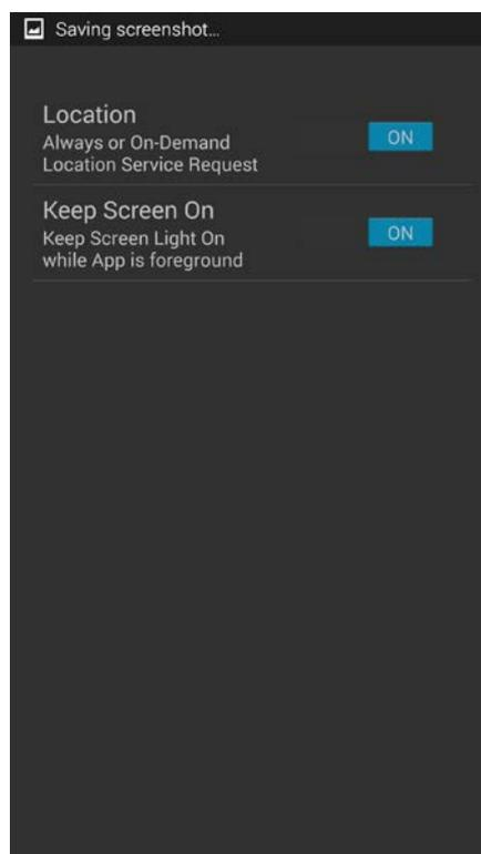
Location Settings: when this option is set, NSG will always request a GPS info from system which increase battery consumption. When it's off, NSG only request GPS when the map is open.
