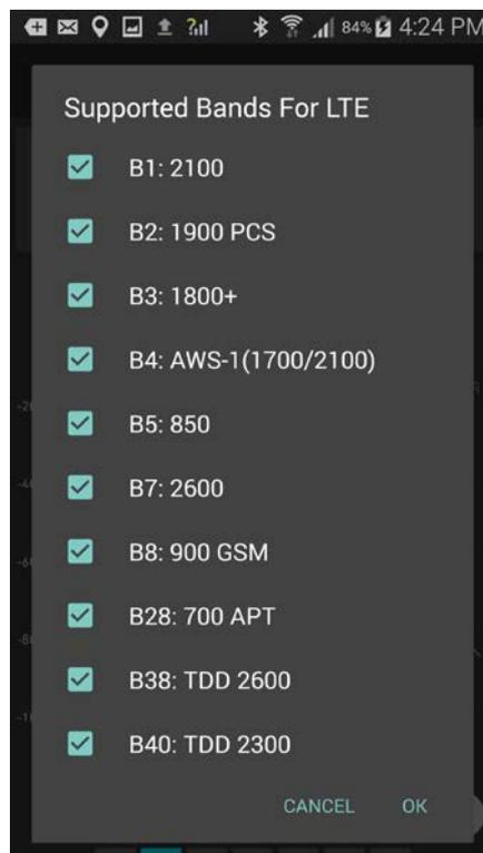
B1: 2100 etc. the device will be locked to the indicated subset of LTE bands.
