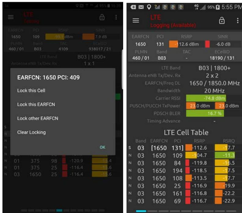
The entity locked on is highlighted in   in the list. To undo a lock action, long-tap and choose Clear locking.
