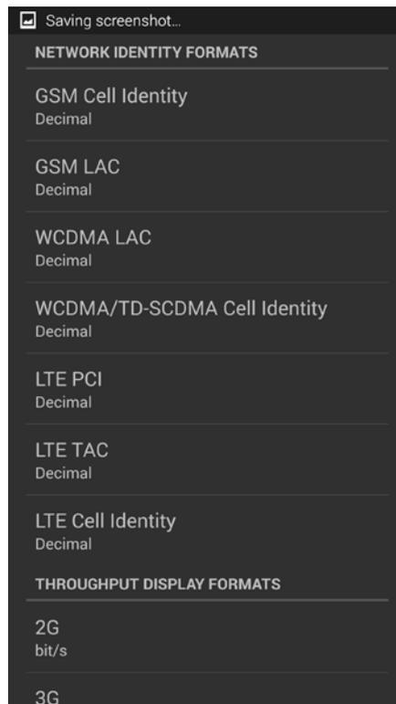
A number of value elements in NSG can be displayed in either decimal or hexadecimal format. In some cases, parameter-specific formats are also selectable (for example, Group ID/Phy ID for LTE PCI). Display format settings take effect when NSG is restarted, both in live mode and during log file replay. They also persist after NSG is restarted.
